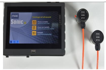
SONIC15 is a device for non Destructive Tests and surveys which uses ultrasonic pulse velocity and sonic tests on masonry with instrumented hammer. It supports extension, too for surveys on foundation piles with P.I.T. methodology. In spite of compact dimension of the unit, there is a wide monitor of 7" with integrated touch screen which allows to use it in immediate and effective way during construction.
